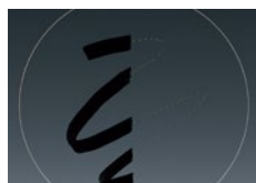
Image illustrates resistance to grime (oil-based felt marker) left side: Without Fluorine Coating right side: With Fluorine Coating
